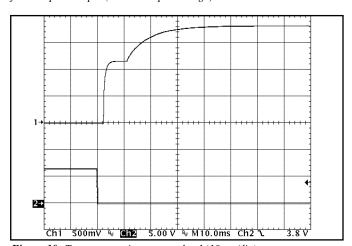
Figure 10: Turn-on transient at zero load (10 ms/div).
