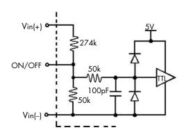
Figure B: Internal ON/OFF pin circuitry
