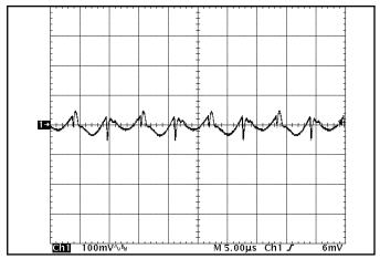
Figure 16: Output voltage ripple at nominal input voltage and rated load current (100 mV/div). Load capacitance: 1µF ceramic capacitor and 15µF tantalum capacitor. Bandwidth: 20 MHz. (See Figure 13)
