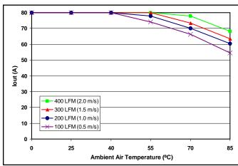
Figure 7: Maximum output power derating curves vs. ambient air temperature for airflow rates of 0 LFM through 400 LFM with air flowing from output to input (nominal input voltage).
