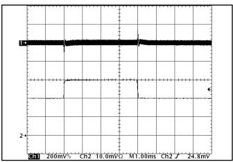
Figure 12: Output voltage response to step-change in load current (50%-75%-50% of lout(max):  $dV/dt = 5A/\mu s$ ). Load cap:  $480\mu F$ ,  $15 \text{ m}\Omega$  ESR tantalum capacitor and  $1\mu F$  ceramic capacitor. Top trace: Vout (200mV/div), Bottom trace: lout (20A/div).
