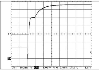
Figure 9: Turn-on transient at full load (resistive load) (10 ms/div). Input voltage pre-applied. Top Trace: Vout (500mV/div). Bottom Trace: ON/OFF input (5V/div)
