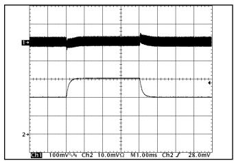
**Figure 11:** Output voltage response to step-change in load current (50%-75%-50% of lout(max);  $dV/dt = 0.1A/\mu s$ ). Load cap:  $15\mu F$ ,  $450 \, m\Omega$  ESR tantalum capacitor and  $1\mu F$  ceramic capacitor. Top trace: Vout (100mV/div), Bottom trace: Iout (20A/div).
