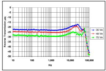
Figure 21: Magnitude of incremental reverse transmission (RT =  $i_{in}/i_{out}$ ) for minimum, nominal, and maximum input voltage at full rated
