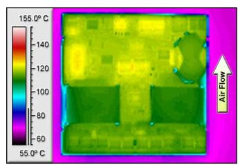
Figure 8: Thermal plot of converter at 78 amp load current with 55°C air flowing at the rate of 200 LFM. Air is flowing across the converter from output to input (nominal input voltage).
