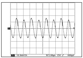
Figure 14: Input Terminal Ripple Current,  $i_c$ , at full rated output current and nominal input voltage with  $10\mu H$  source impedance and  $47\mu F$  electrolytic capacitor (200 mA/div). (See Figure 13)
